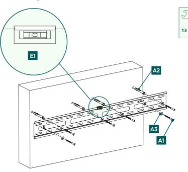
Attach the wall bracket to the wall as shown above using the enclosed mounting material ([A2 plug, [A3] M8 washer, [A1] 8x60 mm screw and [E1] spirit level).
