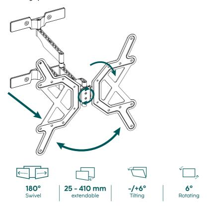
• To adjust the tilt, open the side fastening screws, set the desired tilt and tighten the screws again using the pipe bowl spanner [F1].
