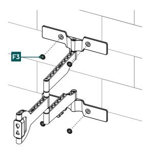
• Then attach the enclosed cover caps [F3] to the hexagon head screws [A1] as shown above.
