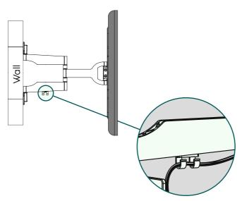
• Stow the cables in the cable holder as shown above.
