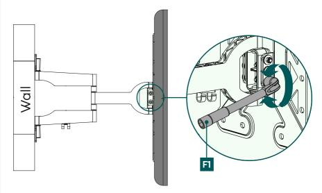
• To adjust the tilt, open the side fastening screws, set the desired tilt and tighten the screws again using the pipe bowl spanner [F1].
