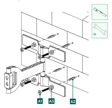
• Attach the wall bracket to the wall as shown above using the enclosed mounting material ([A2] plug, [A3] M8 washer and [A1] 8x60 mm screw).
